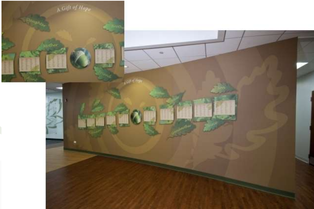
Donor wall highlighting the names of 2011's donors and recipients. The dimensional elements are fabricated with magnetic sheets on cleated Sintra for changeability.
